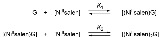
Scheme 5 Equilibria for the complexation between [\text{Ni}^{\text{II}}\text{salen}] and alkaline earth metal ions
